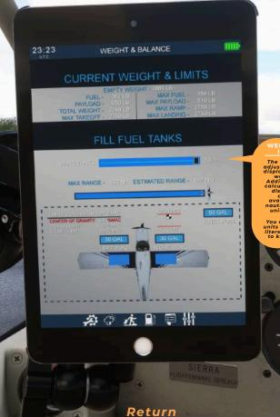
The sliders allow you to adjust the tank levels and display the corresponding display the corresponding weights and limits. Additionally, the system calculates and shows the distance that can be covered with the available or set fuel in nautical miles (nm). Fuel units are measured in gallons.
